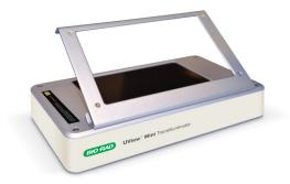
UV shield held in place by the magnets. Shield is also positioned to depress the UV safety switch.
