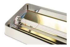
7. Place the top cover back on the device and fix the 4 screws back into the top-cover holes. Check the UV bulb function. Use the UV shield to protect your eyes before turning the power on. If the UV bulb does not work, check whether the bulb is installed properly.
