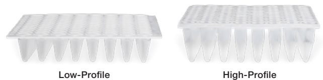
Fig. 1. PCR plate height. Choose between low-profile and high-profile PCR plates based on your PCR instrument's dimensions.
