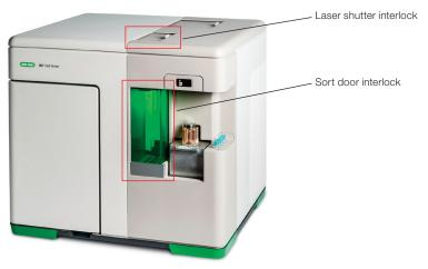
Fig. 10. S3 and S3e safety interlocks.
