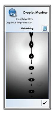
Fig. 37. Droplet Monitor window.
