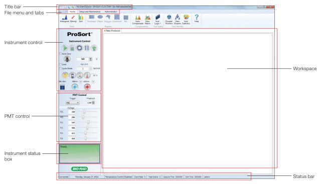
Fig. 13. Main software window for user mode.
