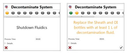
Fig. 130. Decontamination instructions to prepare the system.
