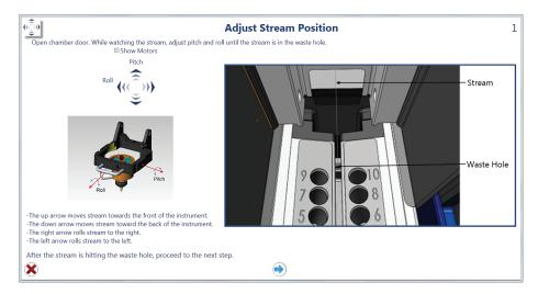
Fig. 121. Adjust Stream Position window.
