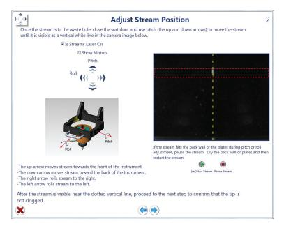
Fig. 122. Adjust Stream Position window.
