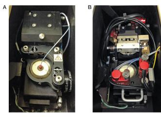
Fig. 8. Nozzle compartment containing the nozzle stage. A, Agilis System; B, AutoGimbal System.
