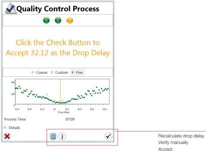
Fig. 40. Drop Delay Alignment Status window.
