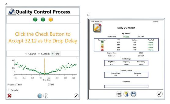
Fig. 36. A, Drop Delay Alignment Status window and B, Daily QC Report.
