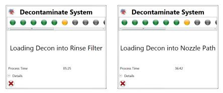
Fig. 133. Decontamination window while priming rinse filter and nozzle path.
