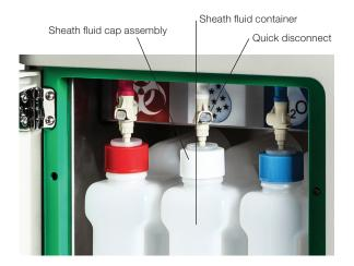
Fig. 4. Fluidics container highlighting the quick disconnect system for the sheath fluid container.
