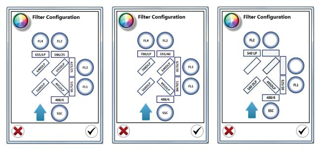
Fig. 68. Different filter configurations. A, 488/561 nm system; B, 488/640 nm system; C, 488 nm system.
