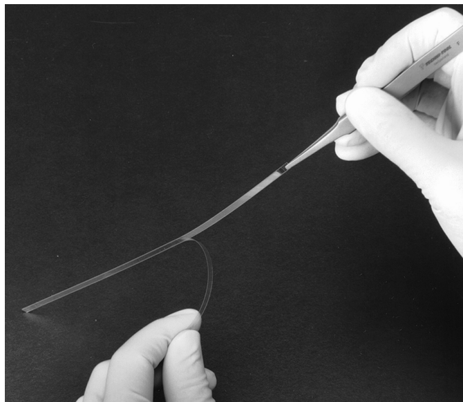
Fig. 3. Removing the cover sheet from the ReadyStrip IPG strip.
