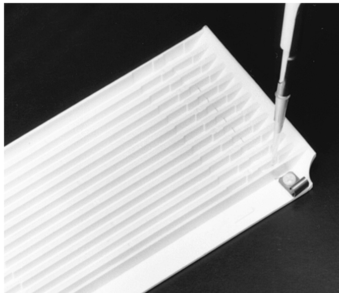
Fig. 6 Wetting the electrode wicks with water.
