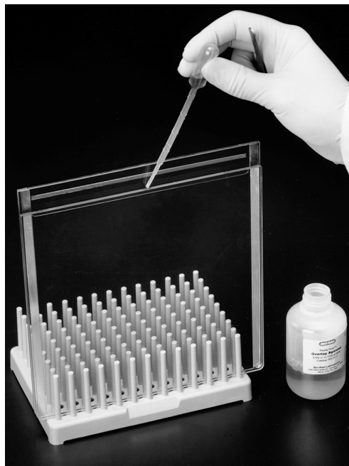
Fig. 12. SDS-PAGE gel with ReadyStrip held vertically in rack. Pipetting overlay agarose into the IPG well.
