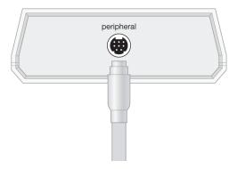
Insert the other end of the cable into one of the peripheral connector ports on the side of the NGC instrument.
