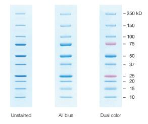
Fig. 1. Comigration of prestained and unstained Precision Plus Protein standards. All standards were run on a 4–20% Tris-HCl Criterion™ precast gel, and the unstained standards were stained with Coomassie Blue.
