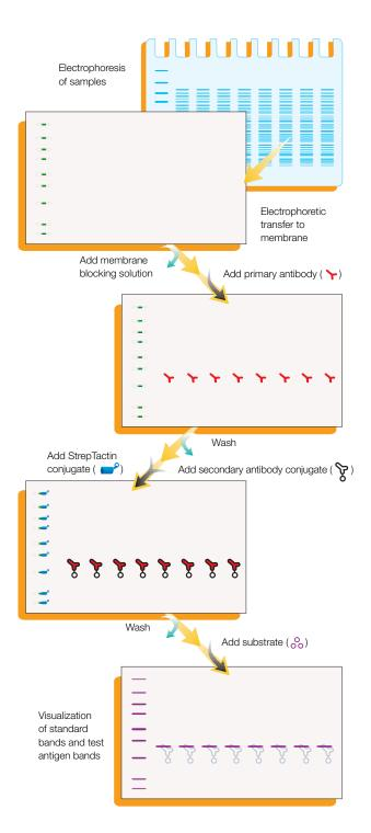
Fig. 3. Summary of Precision Plus Protein standard band detection on an intact blot.
