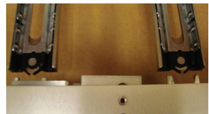
Fig. 17. Replace the drawer. Align the two sets of prongs on the back end of the drawer with black ends of the tracks.
