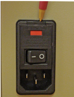
Fig. 18. Replacing the fuse.
