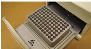
B, Place plate support block in drawer.
